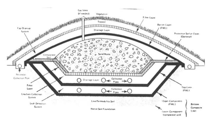
A landfill is a bathtub in the ground, and a bathtub can leak two ways: it can leak through a hole in the bottom (failure of its bottom liner), or it can fill up with fluid and spill over its sides. Either way, it's bad news. The basic problem is the fluid. If a landfill begins to fill up with fluid, the weight of the fluid puts pressure on the bottom of the landfill, increasing the likelihood of bottom liner failure, so any fluid inside a landfill is a potential source of trouble.
