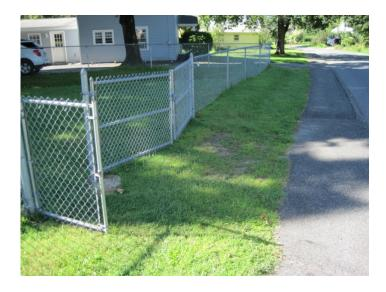
There is no accessible path leading from the sidewalk into the park and the gate to enter the park cannot be opened with a closed fist. An appropriate path should be installed and an accessible latch should be placed on the gate.
