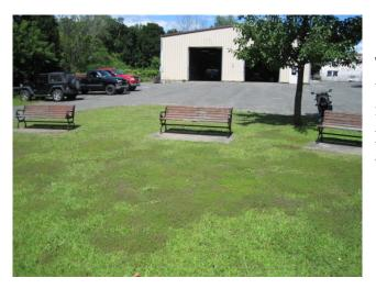
The benches in the park are not connected to the path and did not have an even surface next to the benches for wheelchair access. A proper path should lead to the benches and to adjoining wheelchair access.
