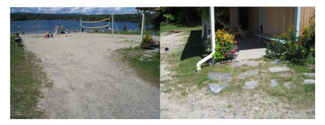
The path leads to the beach where there is no accessible path to the water. A Mobi mat could be placed above the sand to provide wheel chair access down to the water front. In addition, the space leading to the bathrooms (Pic. 2) is rough and leads to a gap. A proper re-pavement of surrounding area is necessary to ensure the bathrooms are ADA accessible.
